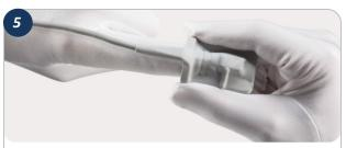
Insert your finger into the probe until it reaches the base of the sensor. The cable should rest on top of your finger, along the back of your hand.
