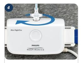
Insert the cannula connection into the device by twisting it into the cannula connection port.
