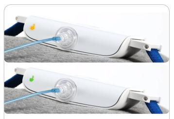
If the device detects a problem with any of the sensors, a flashing yellow icon will appear for 10 minutes. Adjust the sensor that is indicated. The flashing icon will turn from yellow to green and then disappear.
