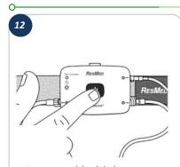
Press and hold the power button until the sensor lights turn off. Once released the study indicator light comes on.
