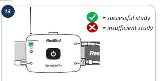
Check that the test complete indicator light is green. This means the test is complete. If the test indicator light is red, please call the support line.
