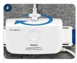
Insert the cannula connection into the device by twisting it into the cannula connection port.
